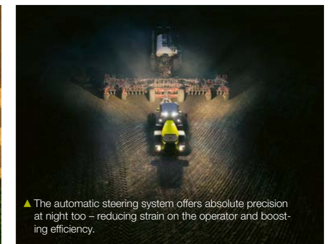
▲ AXION 800 tillage. Digital set-up: GPS PILOT CEMIS 1200 in A-B contour mode and CEMOS.
