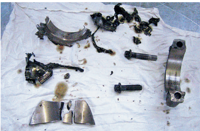
Wrecked connecting rod bearings with fragments of the cylinder liner.
